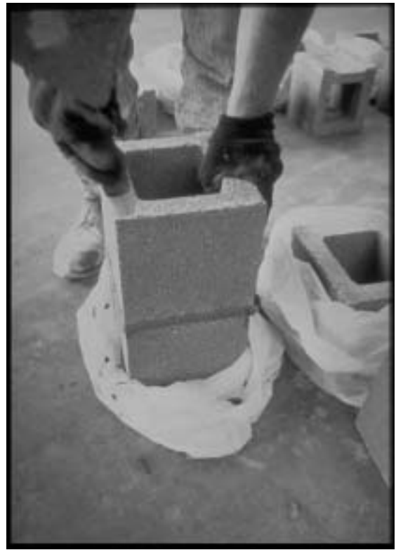
Figure 4—Constructing a Half-Length Prism in a Plastic Bag
