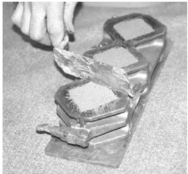
Figure 2—Striking Off Mortar Cube Specimens for Compressive Strength Testing
