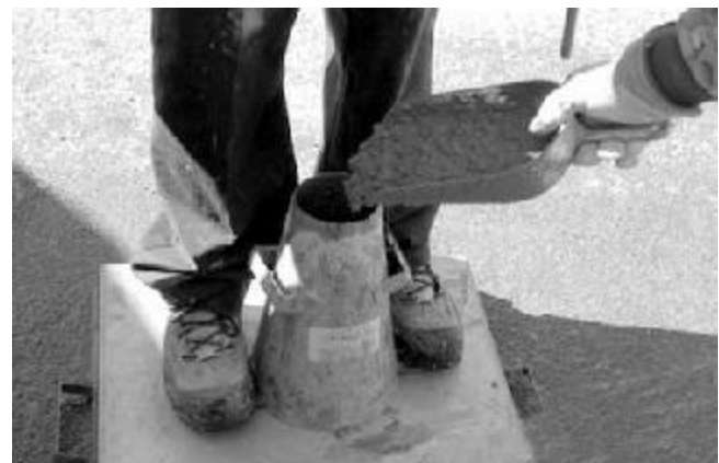
Figure 1—Filling the Slump Cone
