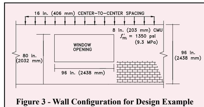
**Figure 3 - Wall Configuration for Design Example**
