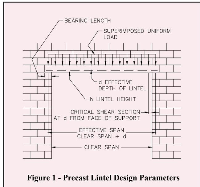
Figure 1 - Precast Lintel Design Parameters
