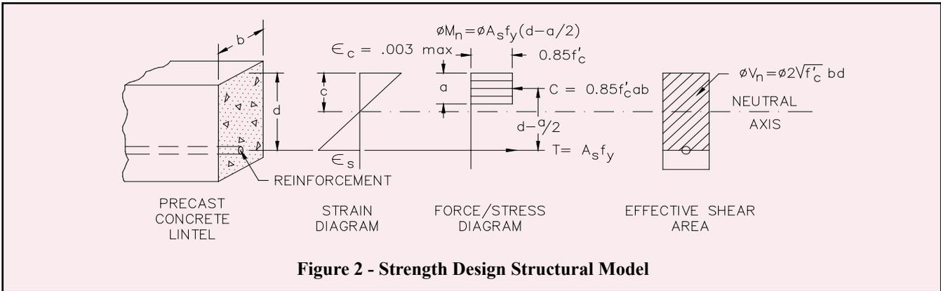
**Figure 2 - Strength Design Structural Model**
