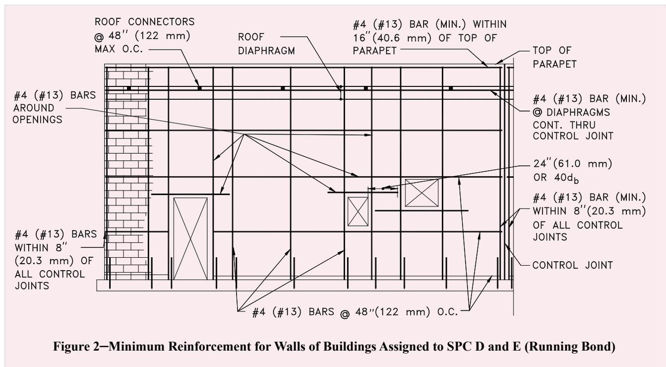
Figure 2—Minimum Reinforcement for Walls of Buildings Assigned to SPC D and E (Running Bond)
