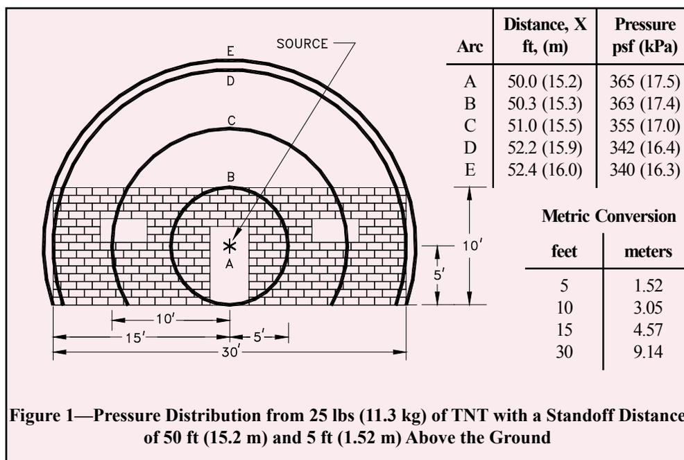
**Figure 1—Pressure Distribution from 25 lbs (11.3 kg) of TNT with a Standoff Distance of 50 ft (15.2 m) and 5 ft (1.52 m) Above the Ground**
