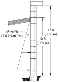
Wall: 12-in. (305 mm) thick concrete masonry foundation wall, 12 ft (3.66 m) high
