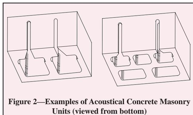
Figure 2—Examples of Acoustical Concrete Masonry Units (viewed from bottom)
