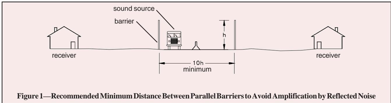
sonry highway sound barriers. For structural design considerations, the reader is referred to *Concrete Masonry Cantilevered Highway Noise Barrier Walls* and *Pier and Panel Highway Sound Barrier Wall Design* (refs. 3, 4).
