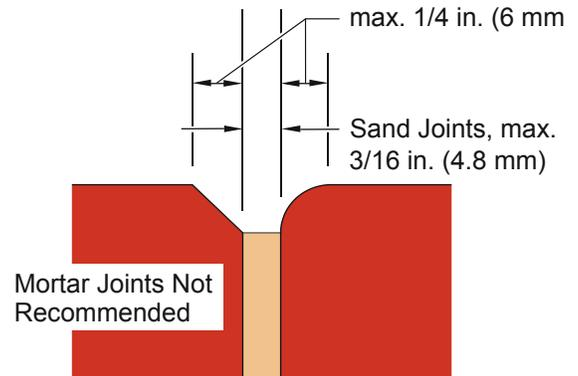
b) Chamfered or Rounded-Edge Pavers
